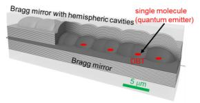
quantum emitter. The open cavity is made of two mirrors brought in close proximity (about 1 micron apart) with the use of dedicated piezo actuators. One of the mirrors has been etched using focus ion beam technology to engineer lattices of hemispheric cavities, which define a photonic lattice. The coupling of the quantum emitters to the photonic lattice modes is expected to result in the emergence of non-classical states of light with spread entanglement [1].
